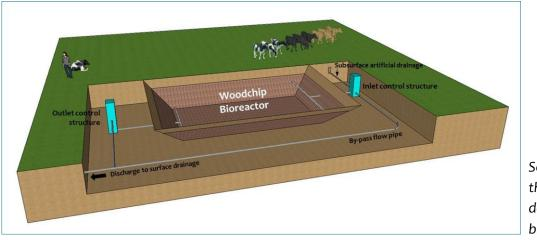
Schematic of the woodchip denitrifying bioreactor
